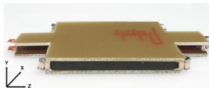
Fig. 1: Prototype of the parallel-plate resonator employed for MRI studies of lithium-ion cells. The B_1 field is oriented along x with B_0 z directed. MRI profiles are generated along y.
