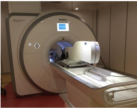
Figure. Set up of CMR-compatible supine ergometer in scanner.
