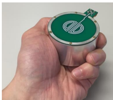
Fig. 1. A small inside-out sensor built with a barrel magnet and a double-D coil.
