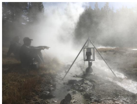
Figure 2. Setup for measuring a depth profile into a biofilm at a runoff of the octopus hot spring in Yellowstone National Park.
