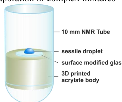
Fig. 1: Sample setup for examination of sessile droplets in 10 mm tubes.
