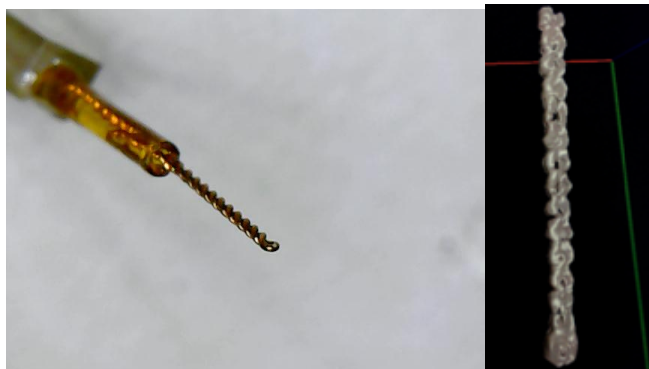
Fig. 1. Left: implantable twisted microcoil with 150 \mu\text{m} copper wire and a total length of 3 mm. Right: MRI image obtained with the microcoil, illustrating the sensitive detection zone of the NMR probe.
