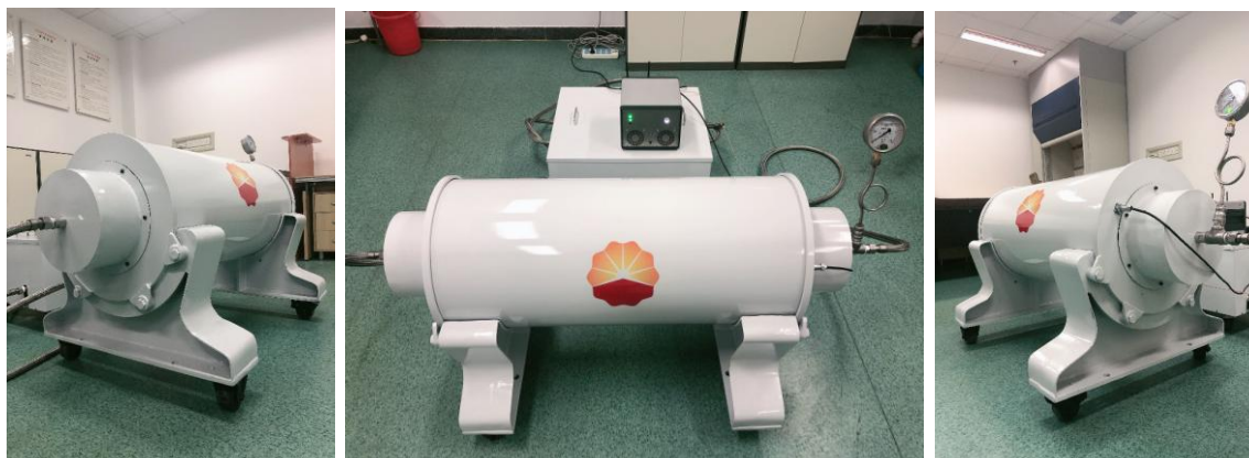
Fig. 1: The photo of NMR multi-phase flowmeter & fluid analyzer.
