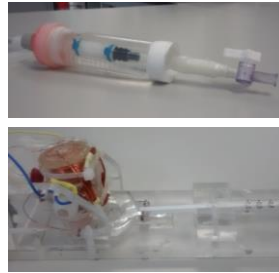
Fig.1. MRI cardiac phantom: the actuator coil with the attached motion sense coil and linkage to the syringe. The syringe and tubing provide a means to fill the chamber with water/lubricant prior to scanning.
