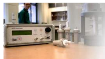
RheoNMR Accessory enabling rheological measurements with NMR
