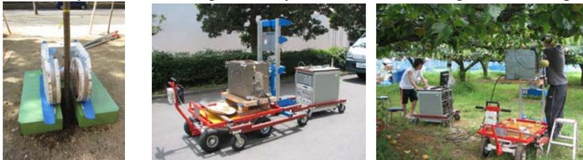
Fig.5 0.2T, 16 cm magnet Fig.6 Mobile MRI (200kg) Fig.7 In-situ measurements
