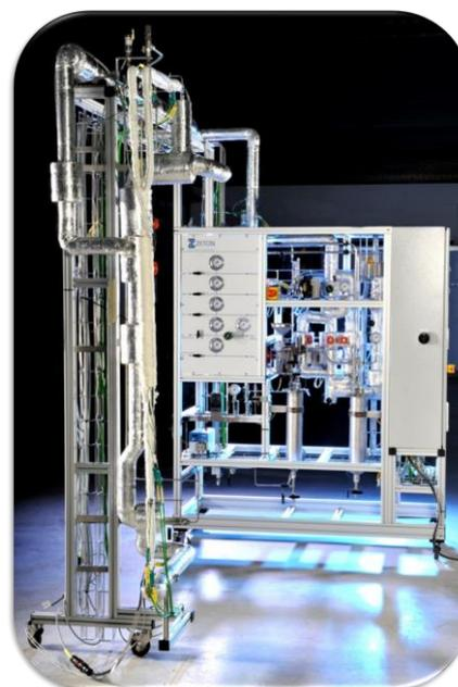
Fig. 1: *Operando* MR reactor capable of 31 atm and 350 °C in up- or down-flow modes of operation whilst inside an NMR magnet.
