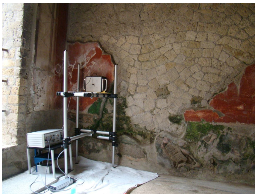
Fig1: Setup of the NMR profiler, illustrating measurements on culture heritage sites. In this particular case self diffusion coefficient is being measured in a mortar layer just below the exterior surface.
