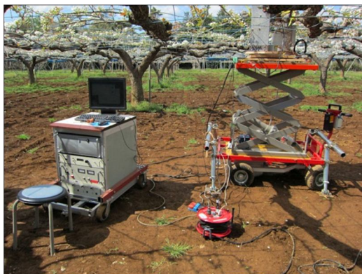
Overview of the electrically mobile and remotely operable MRI system. April,
