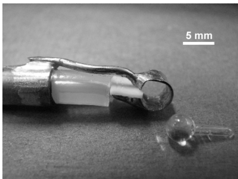
Fig. 1: Photo of probehead with water drop test sample
