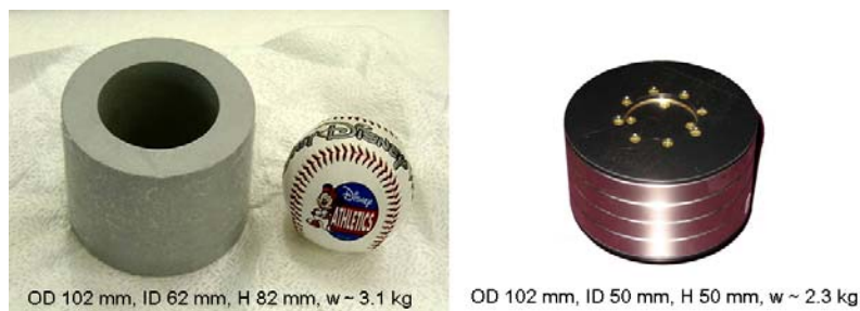
Fig. 1. Two barrel magnets with the same OD.
