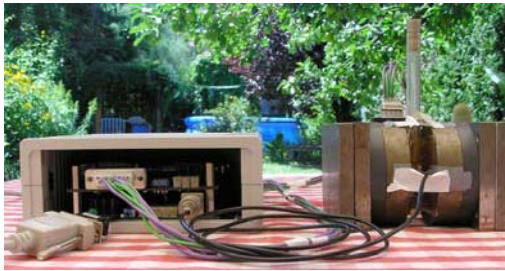
fig.1 Complete nmr imaging machine (without notebook computer) including electronic box (lower board with preamp, receiver, transmitter, gradient D/A, RAM, microcontroller, upper board with gradient power supply and batteries) and magnet.
