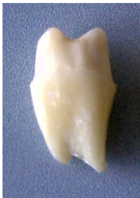
Fig. 1: a prepared human tooth used as a phantom
