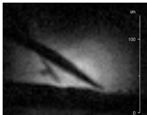
Fig. 2: Slice parallel to the 20 \mu\text{m} surface coil taken from a 3D CTI data set with 3.0 \mu\text{m} isotropic resolution acquired in 58 h and showing glass fibres in doped water.
