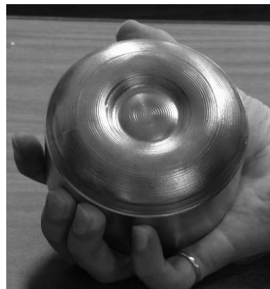
Figure 2: Compact TD-NMR magnet.
