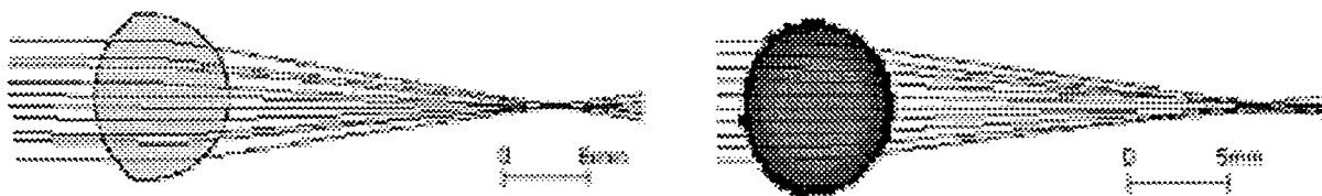
Figure 2: Typical fitted beams and lens surface from optical method (left). Typical ray trace through MRI derived refractive index map (right).
